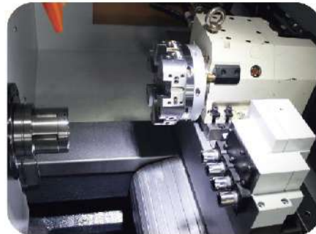
➤ Hydraulic Turret + Face Drilling Device
